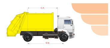
Introduction: In The Rear Loading Compactors Systems, The Unloading Of Containers Is Done Through Hydraulic Winch Or Mechanisms Hydraulically, And Compacted Into The Body By Semi-automatic Process Using Highly Advanced Packing System – These Compactors Are Fast, The compactor is Equipped with safety lamp, Reliable Safe And Yet Economic And It Is Eco-friendly.
